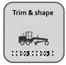
• Initial compaction is followed by the grader to reshape the top course and if necessary, to remove excess material.
